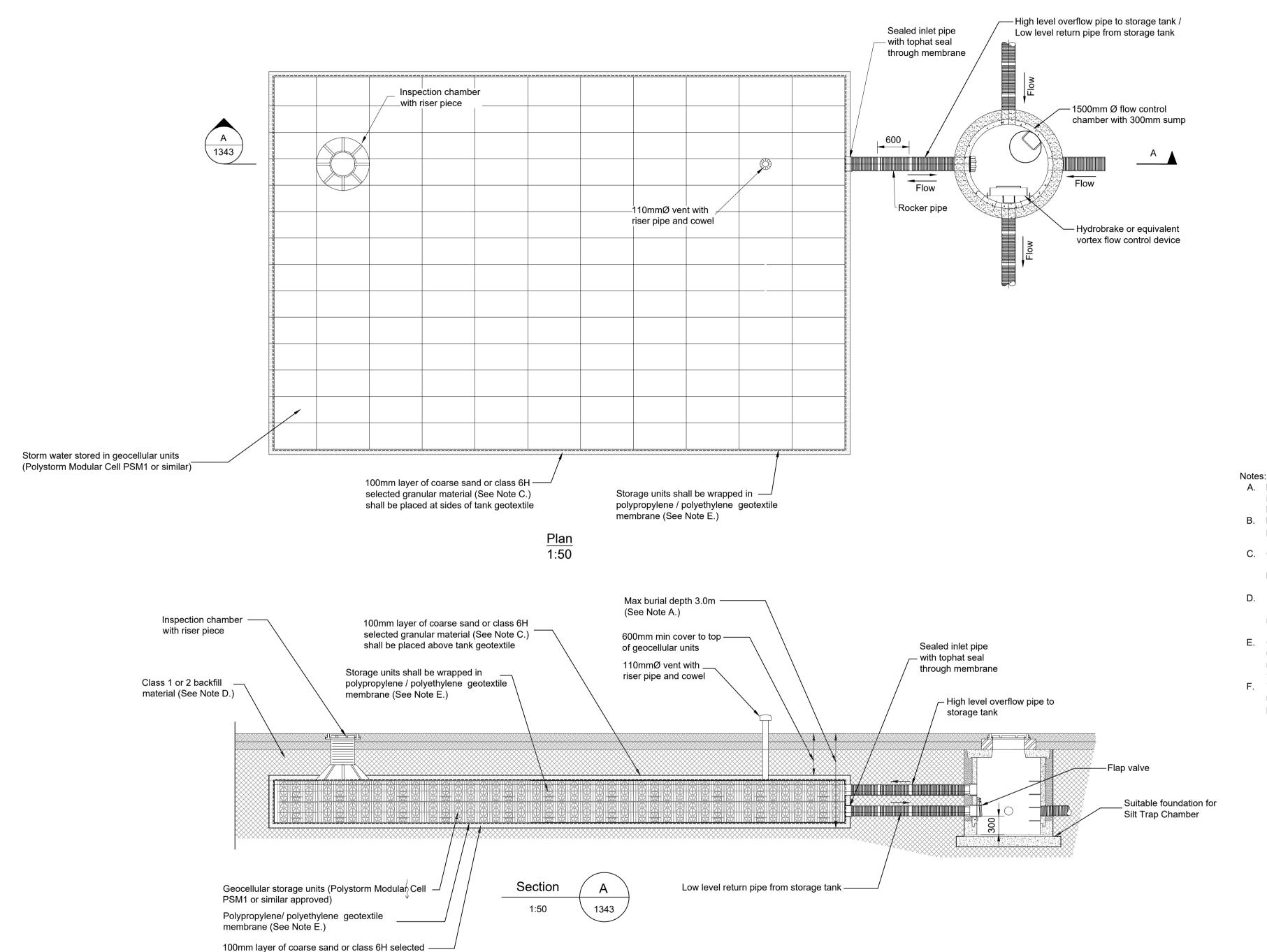
Storm Water Attenuation Tank Details
